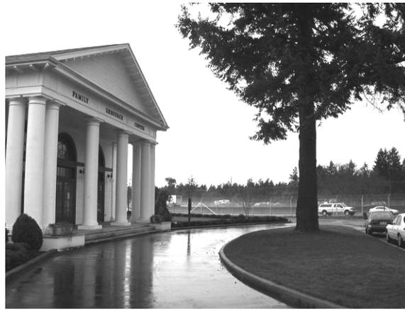
Figure 11. Reduced pavement widths can deter parking along roadways within the standoff (ERDC-CERL 2004).
