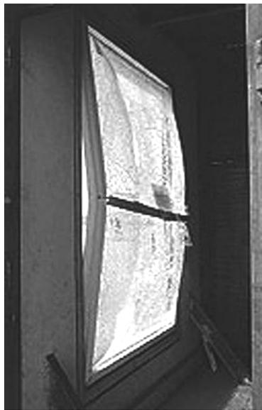
Figure 45. Flexible frame blast-resistant window with collapse mechanism at mid-window (Oldcastle-Arpal, not dated).
