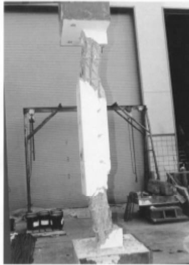
Figure 15. Buckling of an unwrapped reinforced concrete column (Crawford, Malvar, and Morrill 2001).
