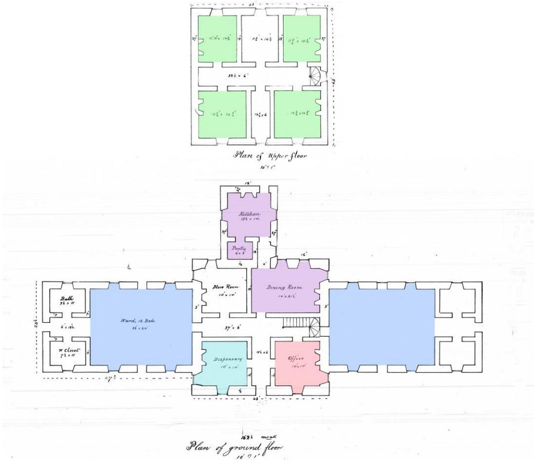
Figure 106. Circular #4 Hospital 2<sup>nd</sup> floor plan [top] and 1<sup>st</sup> floor plan [bottom], 1867 (NARA College Park, RG 77 MISC Fort Files, Fort Bliss).
