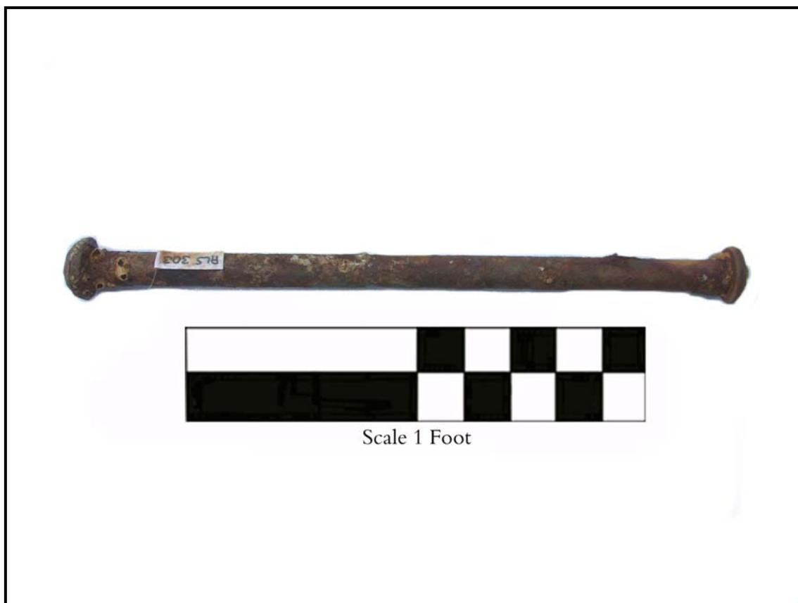
**Figure 48. ALS-303 Fastener with rove.**
