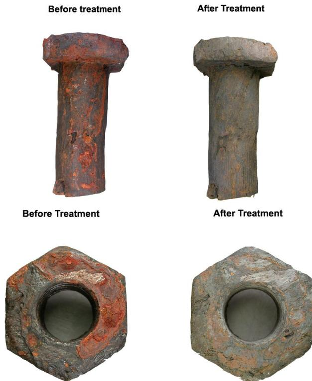
**Figure 2: Spar nut (HL-502) and bolt (HL-511) before and after sub-critical treatment.**
