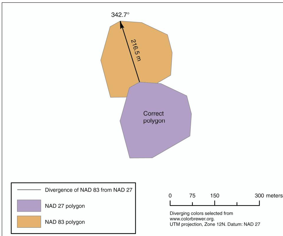
**Figure 3.1. GPS measurements taken with the NAD 83 datum but then projected as if the measurements were collected with the NAD 27 datum (see text for explanation). The resulting error in site location is a standard offset in site location, typically around 200 m.**
