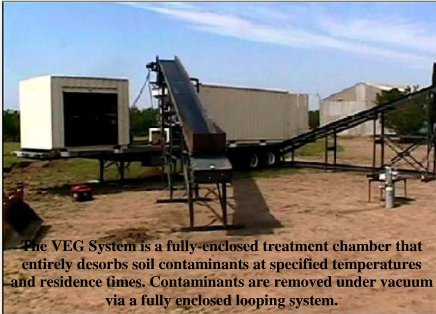
The VEG System is a fully-enclosed treatment chamber that entirely desorbs soil contaminants at specified temperatures and residence times. Contaminants are removed under vacuum via a fully enclosed looping system.
