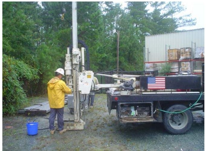
A GeoProbe is deployed to test for contaminants at an IRP site.
