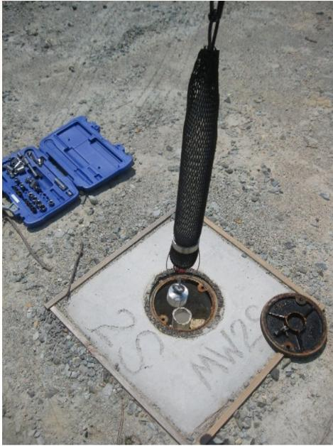
The PDB technique, shown deploying here, uses the principle of diffusion, or the movement of particles from an area of high concentration to an area of low concentration until equilibrium is reached, and replaces purging and low-flow sampling methods in groundwater monitoring wells.
