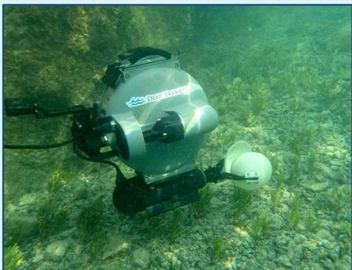
Figure 10: ROVs are being used in Vieques to reduce the dangers of diving on munitions sites, significantly cutting the need for divers and the associated costs. FY14 and FY15 uses include underwater structure inspections, marine ecology surveys, and munitions tracking. Future planned uses include underwater geophysics and sample collection.
