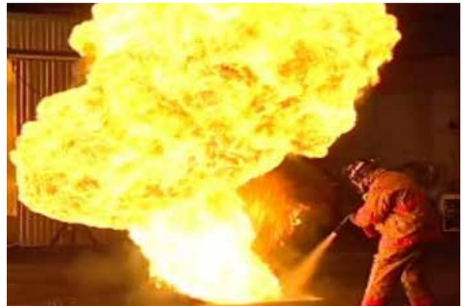
*The Army Test and Evaluation Center performed hundreds of pan-fire tests during the developmental phase of the program.*
