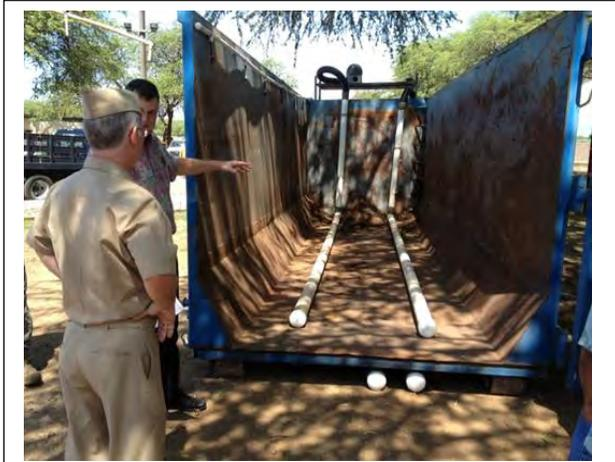
In-vessel composting. Developed at NAVFAC Hawaii as a means to “cook” green waste at temperatures above 140 deg
