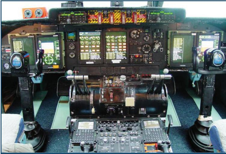
Shown above is the cockpit of the upgraded C-5M Super Galaxy. This aircraft includes the Avionics Modernization Program (AMP) upgrades. The CMC/Wx Radar Modification program upgrades will interface and be presented on the new digital readouts making the workload easier for pilots and crew alike and will provide much more real-time data than previous analog equipment.
