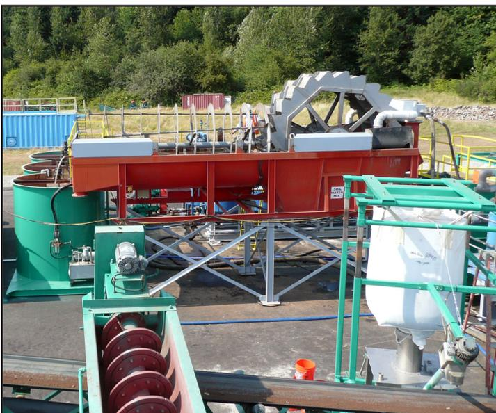
*The multi-stage soil treatment process included a closed-loop water treatment system, allowing all process water to be reused.*
