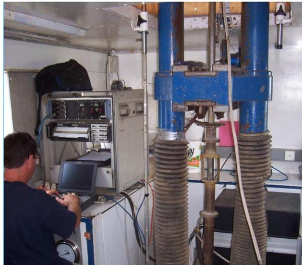
A Laser-Induced Fluorescence Cone Penetrometer provided real-time data analysis to accelerate delineation of the fuel contaminant plume.
