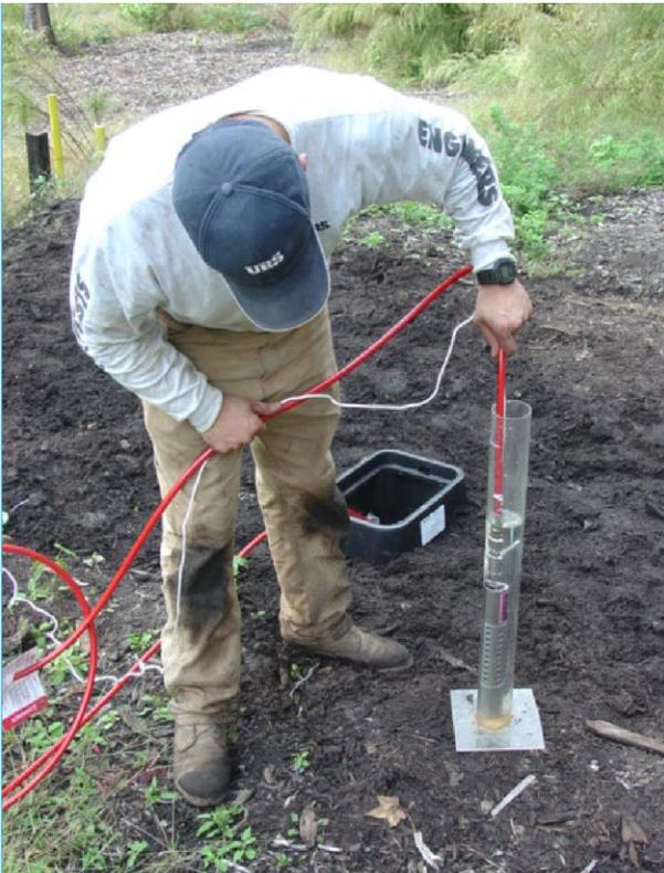
Testing an iSOC infusion device for hydrogen delivery.
