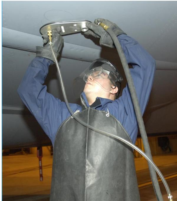
The new "sealvac" bowser unit is used to empty fuel cells and tanks prior to inspection and repair. The unit uses a special adapter plate which essentially eliminates JP-8 fuel spills. Reduced health exposure and reduced safety risks have also been realized.
