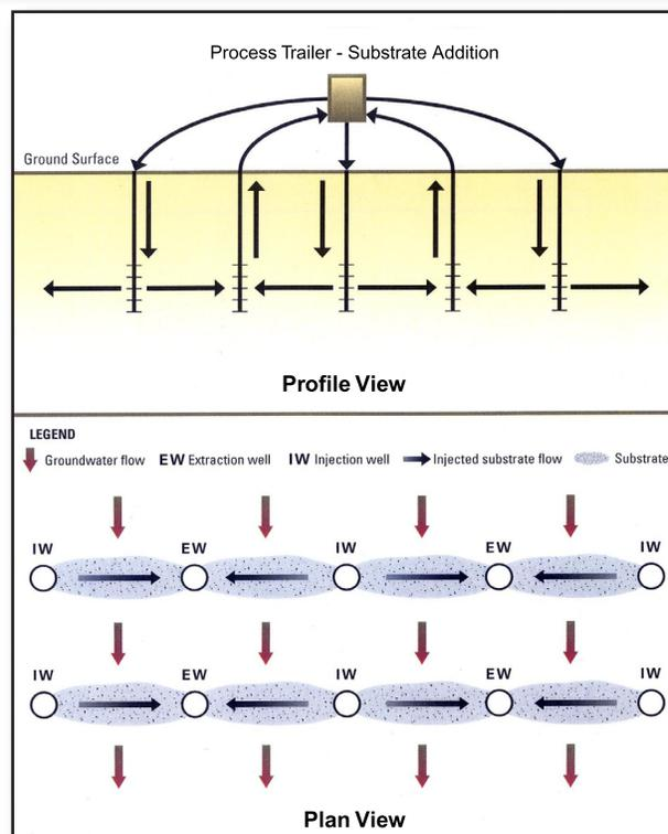
Figure 1. Innovative push-pull delivery technique uses a simple mobile process trailer and generator to inject substrate into the aquifer.
