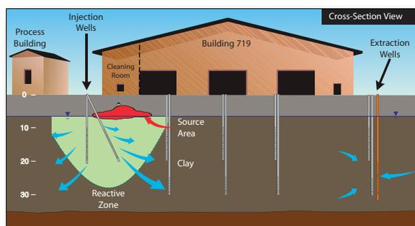
Figure 2: Conceptual Model for Accelerated Anaerobic Biodegradation Recirculation System
