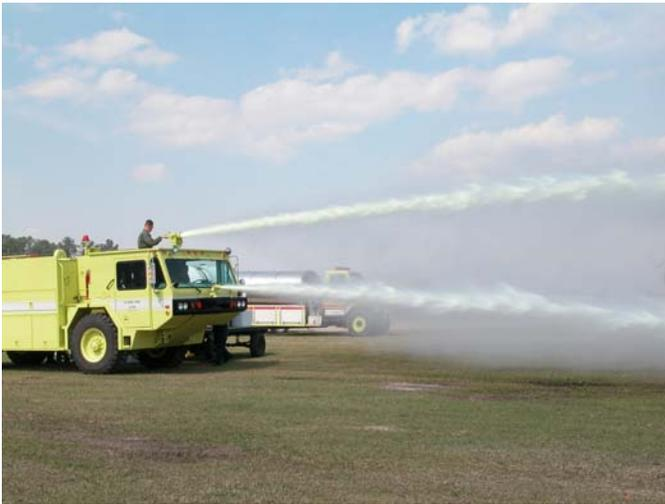
The Aircraft Rescue and Firefighting (ARF) unit on Station is required to test the nozzles on its P-19 "fire trucks" on a regularly scheduled basis. The tests include spraying water and spraying Aircraft Fire Fighting Foam (AFFF). AFFF is an expensive, specially designed chemical foam used by ARF to smother and extinguish fuel fires. Generally, these tests are held on open terrain that runs off into the stormwater system, because AFFF cannot be
