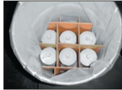
*DNSC took measures to provide redundant protection for the mercury by over-packing the 76 pound flasks in 30-gallon sealed drums.*
