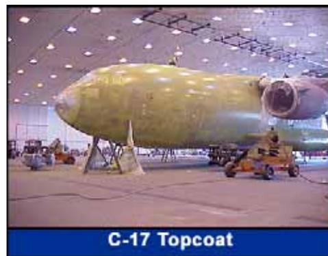
The P2 team collaborated with Air Force Research Lab, aircraft paint vendors and the AF Corrosion Program Office to improve and/or replace previous C-17 aircraft topcoat. This productive teamwork led to a new topcoat, the Advanced Performance Coating, being used in C-17's. The AF realized a \$115 million life cycle cost savings due to improved durability.
