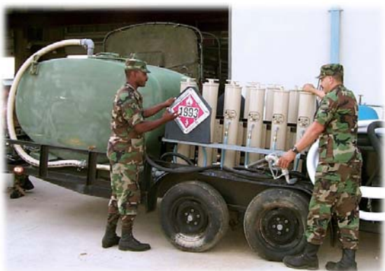
The diesel fuel recycler has allowed the TXARNG to recover 3,100 gallons of diesel fuel, for a reduction of 15.9% and cost savings of $14,500.
