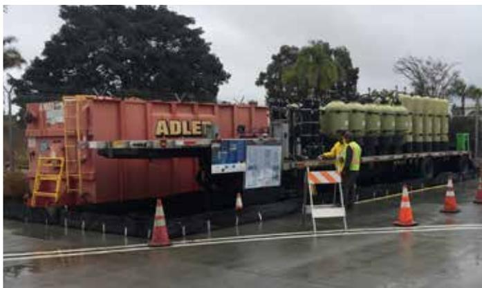
MCAS Miramar EMD staff employ their mobile trailer-mounted treatment system to remove PFAS contaminants from AFFF-impacted wastewater. Water is processed through the system vessels of organoclay, granular activated carbon, ion-exchange resin media, and colloidal scavenger resin. After sampling, staff discharge the wastewater to the sanitary sewer.
