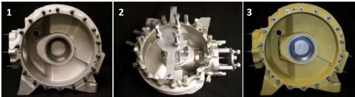
**Figure 1:** Example AH-64 Tail Rotor Gear Box in the blasted condition (1), after the application of custom-designed masking agents (2), and after the application of Tagnite (3).
