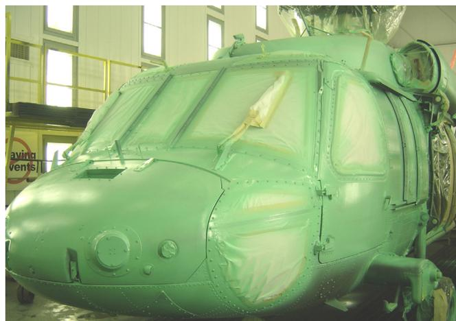
*Hazardous hexavalent chromium (Cr6+) primer on the interior and exterior of aircraft have been replaced with non-chrome alternatives through targeted identification and risk mitigation processes. Replacements eliminate exposure risks for operators and maintenance personnel.*
