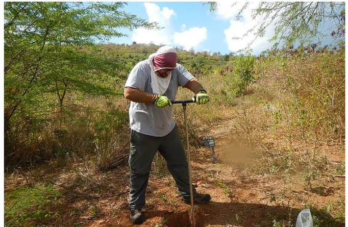
*Subsurface soil sampling beneath a munitions item that was located by an advanced geophysical classification (AGC) technology. The AGC technology allows users to rapidly identify sampling locations, expedite the remedial investigation, and lower costs. Accumulated savings from this use of AGC are estimated to be \$100,000.*
