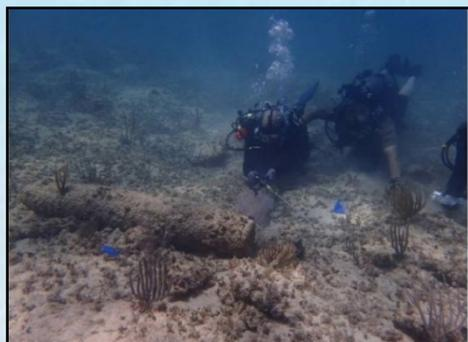
Figure 9. Divers collecting sediment pore water samples adjacent to an underwater munition.
