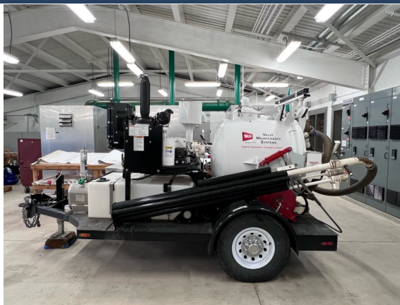
The water utility valve maintenance trailer used at TYAD for water supply repairs.
