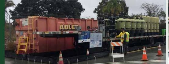
MCAS Miramar Environmental Management Department staff employ their mobile trailer-mounted treatment system to remove per- and polyfluoroalkyl substances (PFAS) contaminants from wastewater impacted by aqueous film-forming foam. After treating the water and sampling it to ensure the system adequately removed PFAS contaminants, staff discharge the wastewater to the sanitary sewer.
