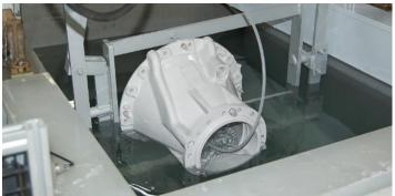
The Tagnite anodizing immersion application developed by the Tagnite Technical WG reduces exposure to carcinogenic hexavalent chromium. The capability extends the life of magnesium components and alleviates regulatory challenges.
