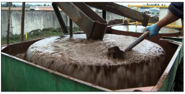
The gravity separation process shown here utilized recovered goldplacer mining equipment to remove the bullets.
