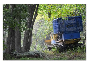
Forest wide herbicide application using a modified skidder. Note the nozzles blasting herbicide mist from the back sides of the skidder.
