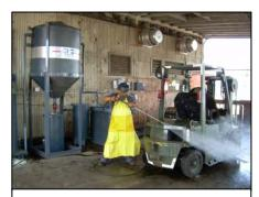
Vehicle wash water recycling system in action.
