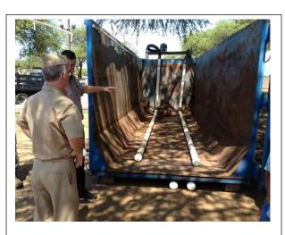
In-vessel composting. Developed at NAVFAC Hawaii as a means to "cook" green waste at temperatures above 140 deg
