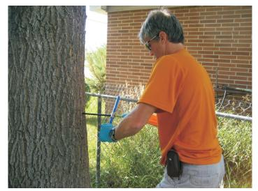
Using tree cores to determine the presence of TCE in the groundwater yielded quick results and saved tens of thousands of dollars over conventional investigations.
