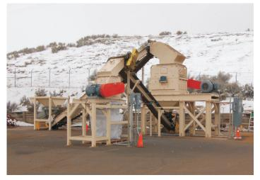
This hammermill crushed cast-iron dummy bombs collected from the Utah Test and Training Range for use as reactive agent for Permeable Reactive Barriers.
