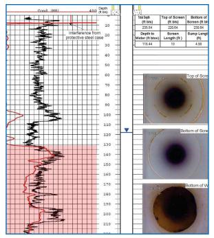
**Monitoring Well MWQ2 Study Summary** This image displays the results of both the geophysical and camera portions of the study for background well MWQ2. Camera images depict screen slots in the well. The geophysical graph displays the red conductivity output that shows the change in aquifer at 130ft.
