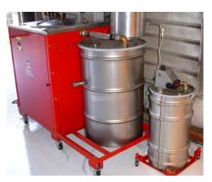
Kleen Paint Gun Cleaner to be used again. The residue, consisting of paint solids, is a fraction of the original waste thinner volume which saves on thinner costs, waste costs, and significant waste minimization is achieved. At the current waste paint sludge generation rate by DynCorp, the Air Station will save approximately \$26,920 per year in sludge disposal and virgin solvent purchases.
