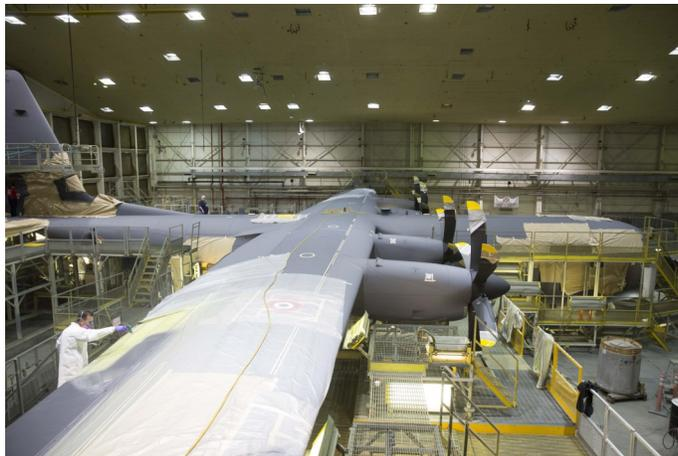
*A C-130J in the Paint Crib where the new Solvent Borne Non-Chrome Primer is applied.*
