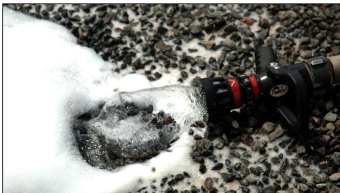
This firefighting nozzle is an efficient means to dispense AFFF which is an effective fire extinguishing agent but the fluorinated compounds can seep into drinking water sources.
