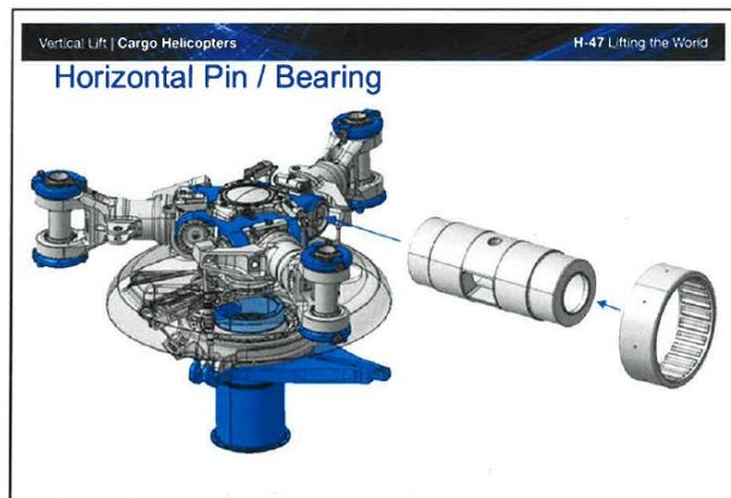
CH-47F Block II IRS Horizontal Pin.
