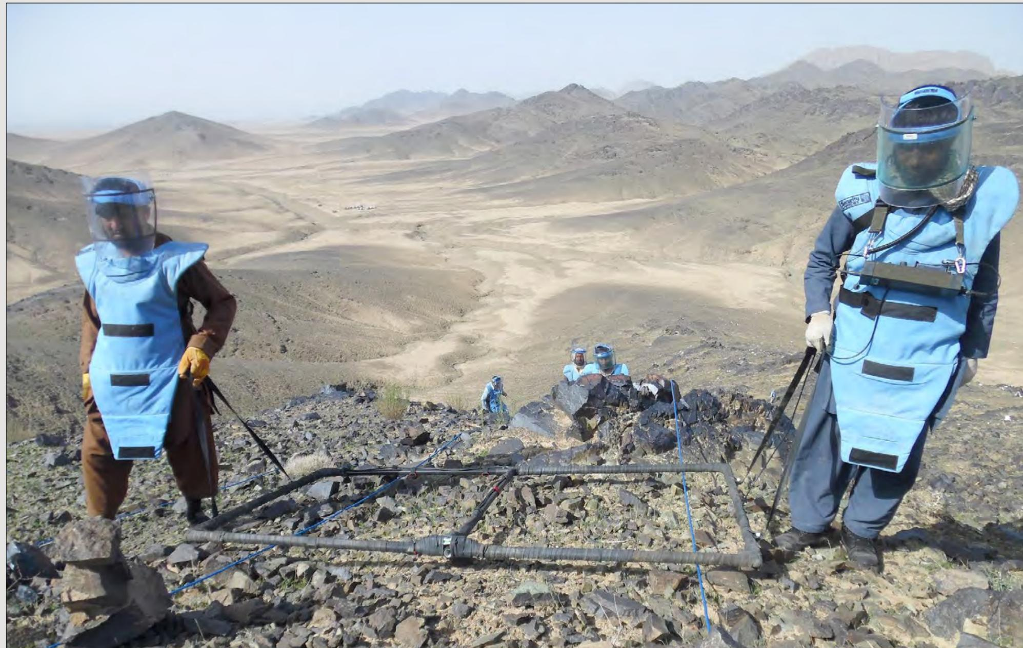
Field personnel perform Digital Geophysical Transect surveying in Afghanistan, March 23, 2015, after a surface clearance had been completed. (Photos courtesy U.S. Army)
