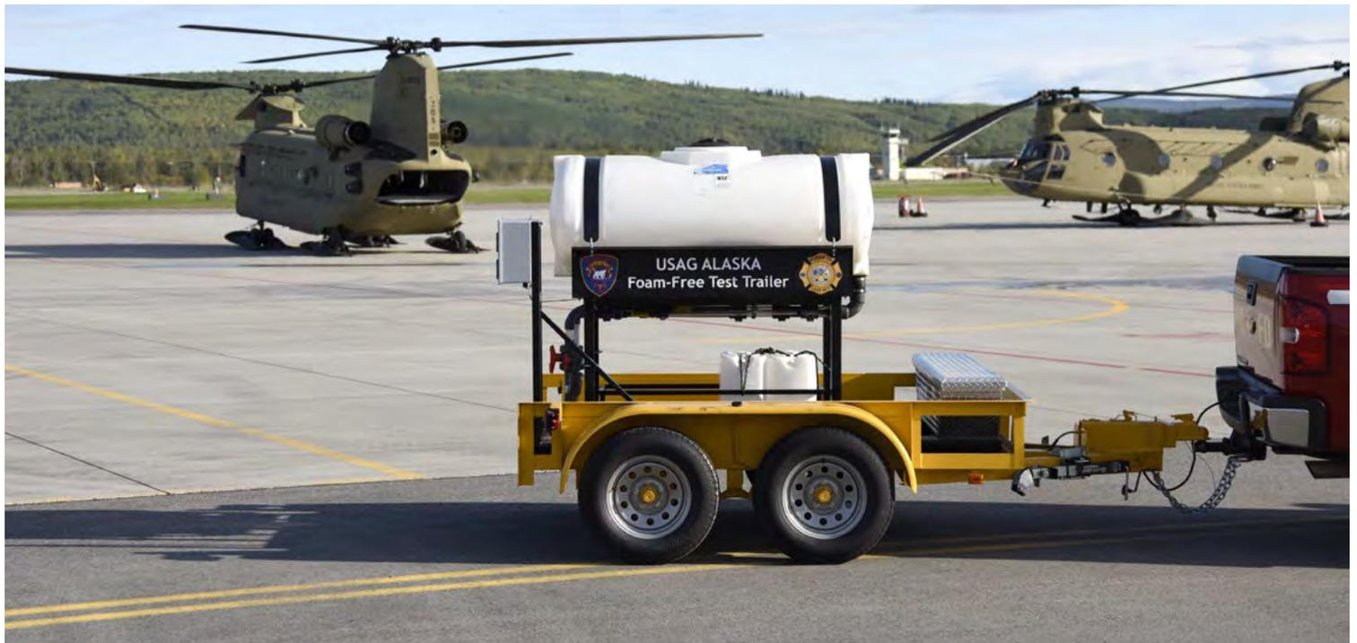
*The foam-free test trailer will be used to ensure that fire trucks and pumpers designed to respond to aviation fuel fires are functioning at their peak, while being protective of the environment.*
