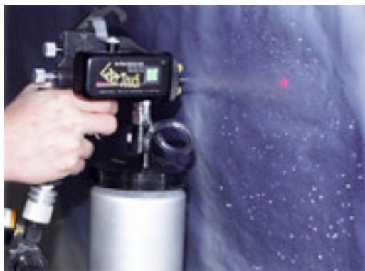
Naval Aviation Depot North Island, California, is using the Laser Touch paint gun to paint aircraft.
