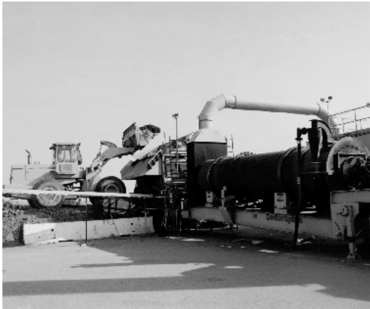
*The Marine Corps/Navy treats fuel-contaminated soil at Tustin Marine Corps Air Station using a portable thermal desorption unit.*
