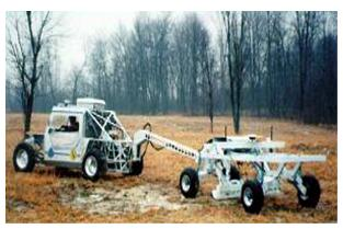
Multi-Sensor Towed Array Detection System is an example of the newer generation of vehicle towed systems.
