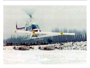
Helicopter-borne detection systems are emerging as a cost-effective tool for characterizing large areas.
