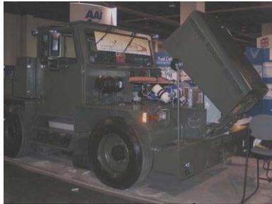
**Hydrogen Fuel Cell Powered Tow Tractor.
